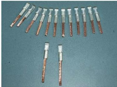
Crimp a Powerpole contact on to one end of each of the cut pieces of wire. Tin the rest of each piece. The solder may be flowed into the contact as well but be careful not to get too much in as it might flow onto the contact surface which is not desirable at all as it will increase the contact resistance of the contact.
