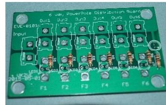
Next take the 6 small LEDs. Place them into the board in the LED1 to LED6 positions. Note that the longer lead is the positive and must go into the hole marked +. Depending on the batch of LEDs, the flat may or may not align with the flat marked on the board overlay. Push the LEDs flat to the board, turn over and solder them in place.
