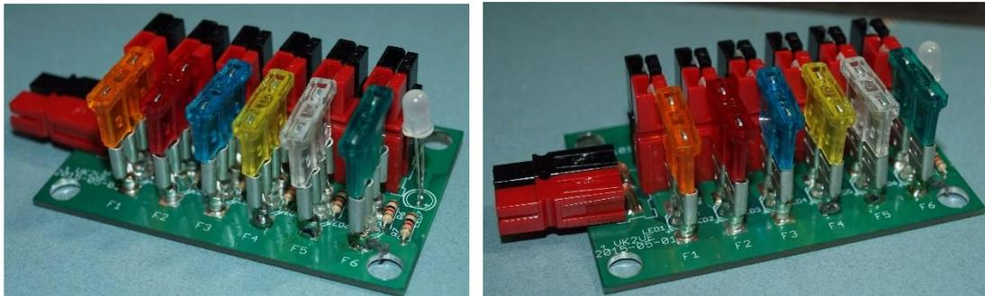
Now take the Powerpole with the long leads. Bend the leads at 90 degrees so that the Powerpole will sit down onto the board with the leads going through the board and the red (+) side towards the fuses. Turn over, solder and trim. If you wish to connect cables directly to the input, rather than the Powerpole, omit this step and solder the input wires into the + and - holes instead.
