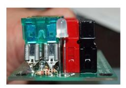
Your board is now complete and you can test it by connecting 12Volts DC power to the input connector. The polarity LED should come on Green. If the polarity of the input is reversed it should light up Red. If this is wrong you may need to remove the LED and turn it around.
