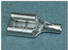
Push a contact onto each blade of each of the fuses. This will be used for the installation onto the board later. Make certain that they are both in the same direction on the fuse as otherwise the fuses will end up at an angle.
