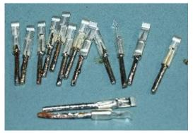
Crimp (or solder) a Powerpole contact onto one end of each of the cut pieces of wire. Tin the rest of each piece. The solder may be flowed into the contact as well but be careful not to get too much in as it might flow onto the contact surface which is not desirable at all as it will increase the contact resistance of the contact.
