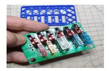
Position jig over parts so that they are aligned properly (several minutes of fiddling)!
