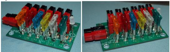
Take the remaining Powerpole with the long leads. Bend the leads at 90 degrees so that the Powerpole will sit down onto the board with the leads going through the board and the red (+) side towards the fuses. Turn over, solder and trim.
