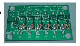
Now you will install the Powerpole connectors and the Fuses. Note that soldering the Powerpole connectors and fuses will require a very hot soldering iron as there is quite a bit of copper around them.
